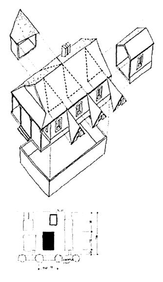
Fig. 8. Axonometrics of modular houses for infill sites showing options that can be added to the basic shell (from the Housing Futures Institute Infill Housing Manual).
