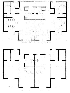
Fig. 7. The same modular shell can be manufactured for three-bedroom townhouses or one-bedroom apartment (Housing Futures Institute).
